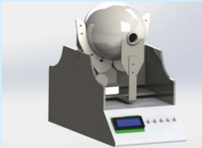
Students have designed Ambu Vent, a low cost automated resuscitator that provides ventilator functionality in emergencies when no other options are available.
