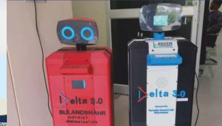
Mr. Nishant Sharma, 3rd year CSE student has created a robot named Delta 3.0 for automatic dispensing of medicines and sanitizers
